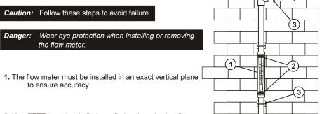
2. Use PTFE tape (or similar) on all pipe threads. Acrylic and other exotic plastics cannot tolerate PVC Glue and/or pipe dope. Even fumes can cause crazing. If you are installing your flow meter to a glued pipe installation, install the flow meter after all glued fittings are dried and lines are purged of all fumes. Never hold the meter with pliers or like tools. DO NOT **OVER-TIGHTEN!**
